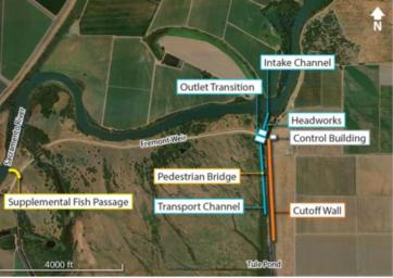
47. As stated in the EIS/EIR, a cutoff wall "is a structure that uses a slurry or cement mix to create a 'wall' along a levee to prevent seepage under the levee or address other levee stability and seepage concerns." (EIS/EIR at p. 2-12.) Later in the EIS/EIR, the cutoff walls and underseepage are explained in more detail:
