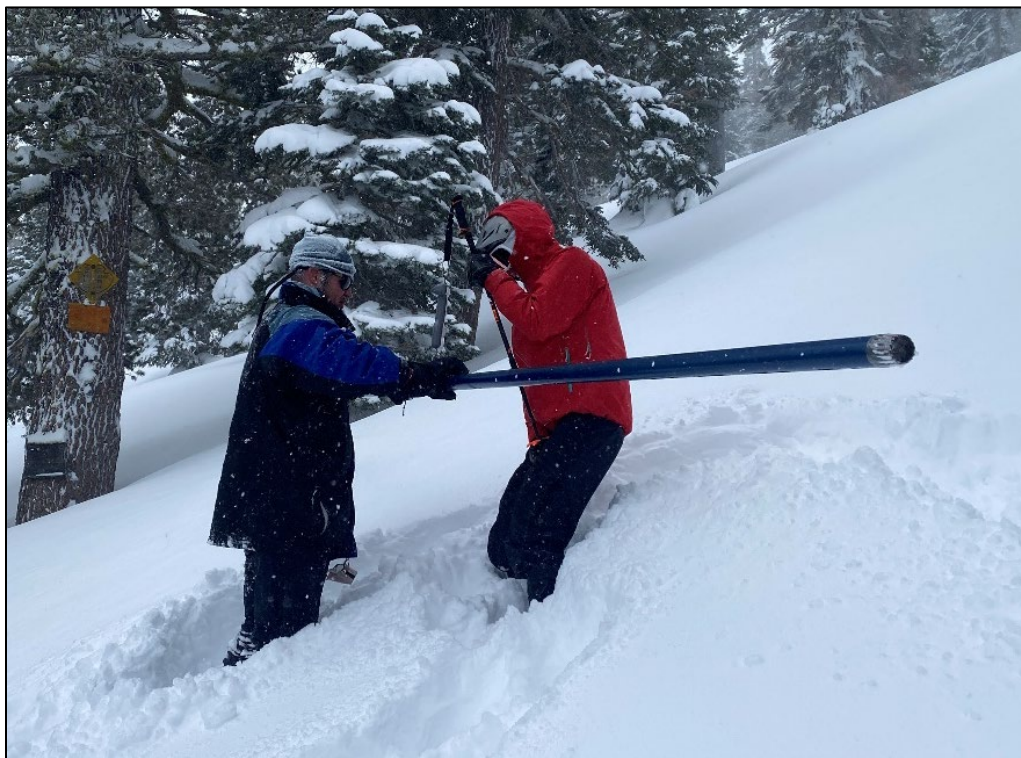
NRCS Snow Surveyors Valerie Bullard and Evan Smith sampling Rubicon #1 snow course in CA Photo by Jeff Anderson, NRCS Snow Survey Nevada
