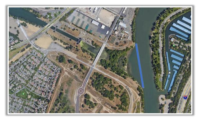
Approximate length of 3,000 cfs flat plate fish screen at confluence of Ship Channel and Sacramento River using actual river bathymetry data.
